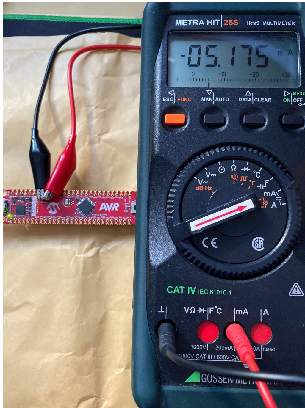
Figure 3-1. Current Reading with Multimeter Setup
