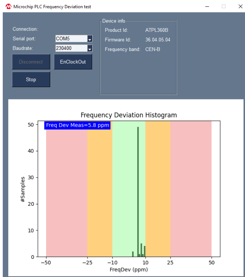
Figure 6-1. Microchip PLC Frequency Deviation Test – Measurement
