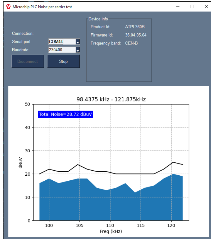
Figure 5-5. PLC Noise Per Carrier Tool Screen Results
