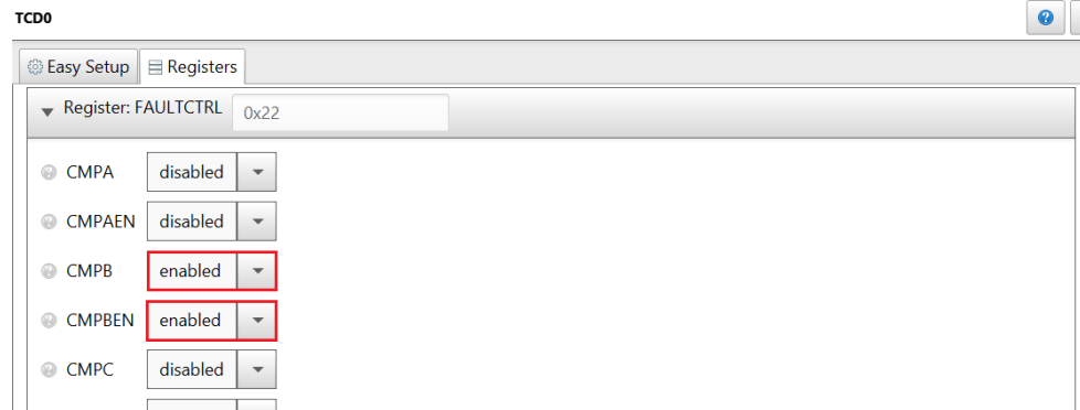
Figure 2-18. TDC0-Registers-CMPB and CMPBEN
