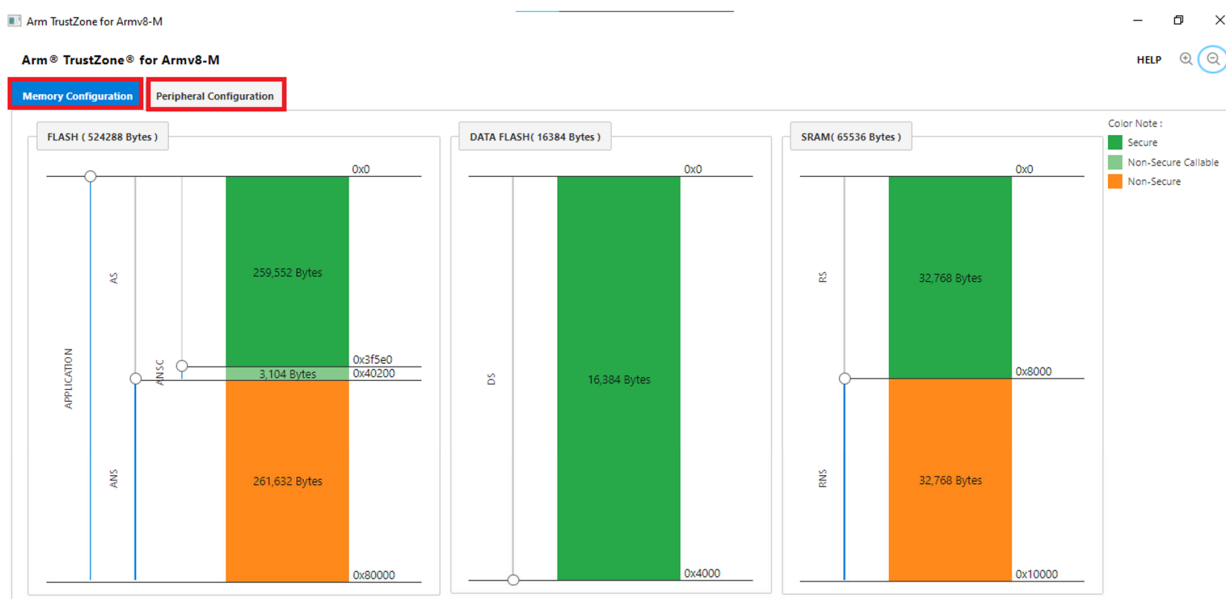
Figure 2-19. Arm TrustZone for Armv8-M
