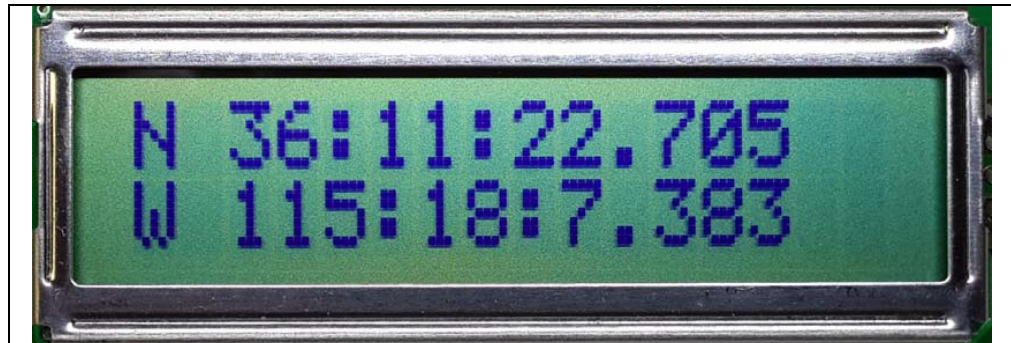
FIGURE 2-5: GNSS Position Display Page.
