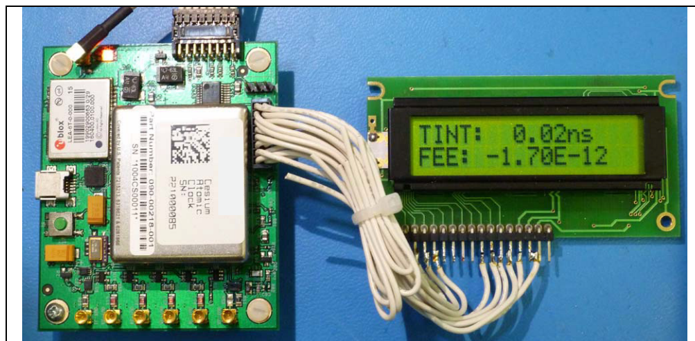
FIGURE 2-2: LCD Display Connection.
