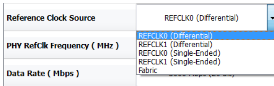
Figure 3-3. SerDes Reference Clock Using the High Speed Serial Interface Generator
