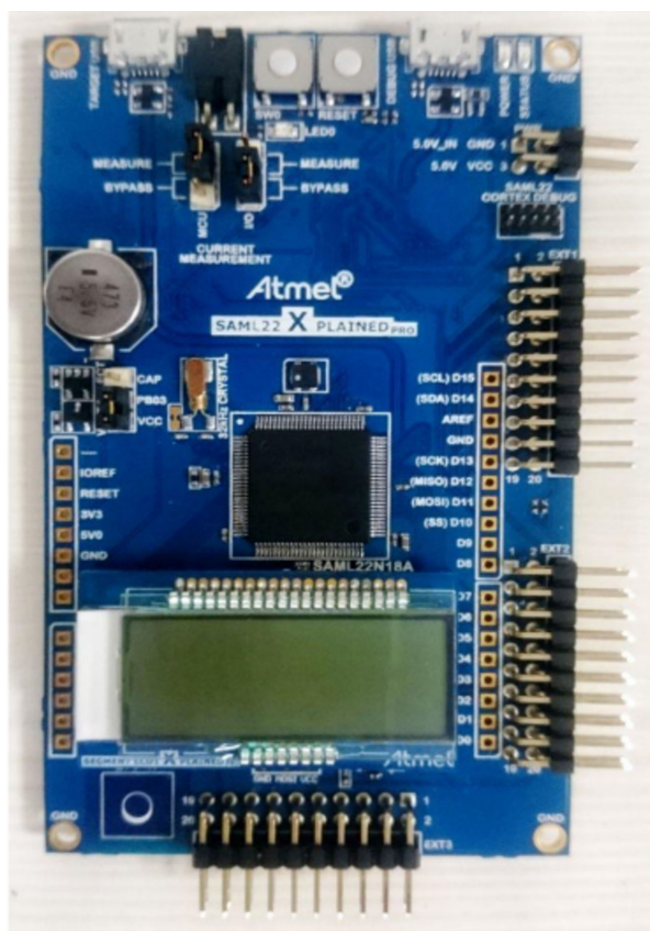
Figure 3-4 SAM L22 Xplained Pro with Segment LCD1 Xplained Pro Board Connection
