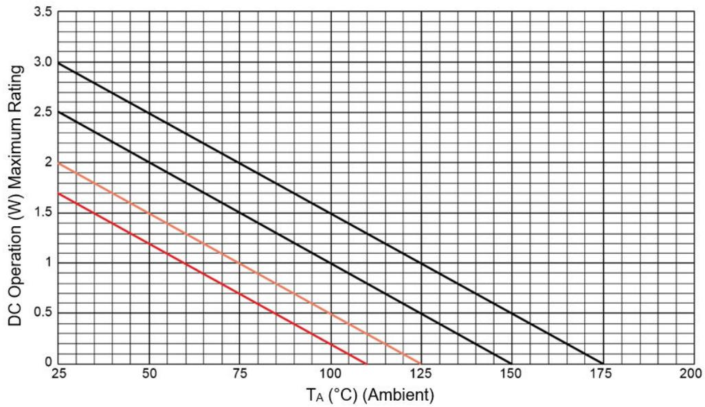
Figure 3-5. Steady-State Derating Curve for Free-Air Mounting ( $R_{\theta JA} = 50\text{ }^{\circ}\text{C/W}$ )
