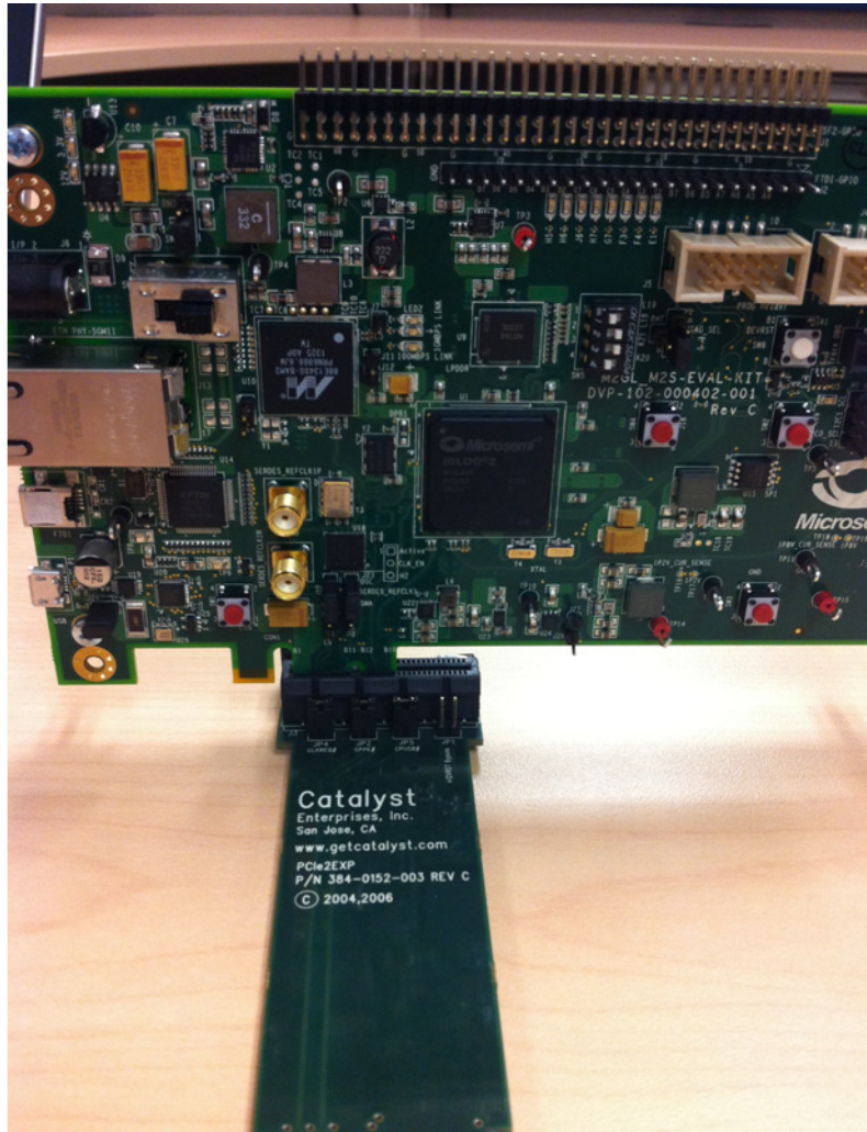
Figure 39 • Inserting the IGLOO2 Evaluation Kit PCIe Connector
