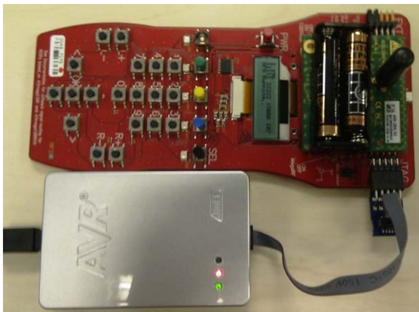
Figure 4-5. Atmel JTAGICE3 connect with key remote board.
