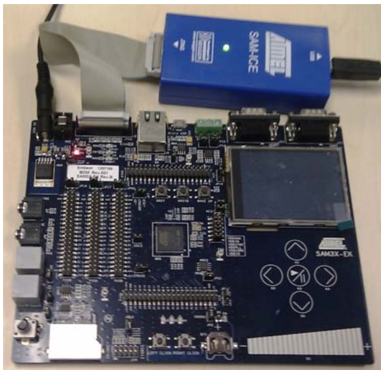
Figure 4-2. SAM-ICE connected with SAM3X-EK.
