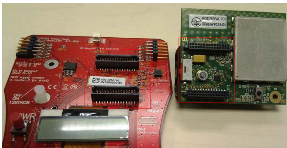
Figure 4-6. Attached light with LED board to key remote board.
