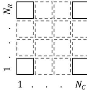
Keys in the touch panel are arranged in a grid format. This touch panel has  $(N_R)$  number of rows and  $(N_C)$  number of columns, forming a rectangular grid of  $(N_R * N_C)$  sensor keys in total.
