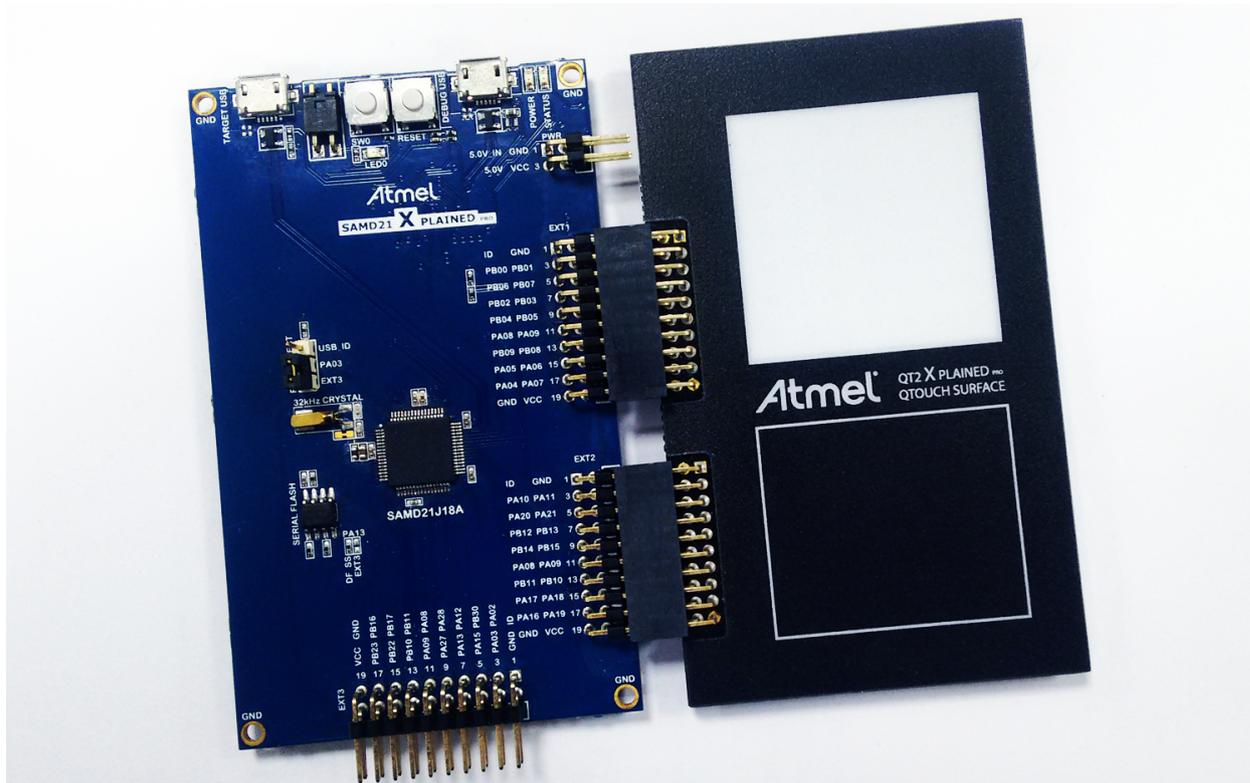
QT2 Xplained Pro kit is an extension board that enables the evaluation of a mutual capacitance touch surface using the Peripheral Touch Controller (PTC) module. The kit provides a 4 by 4 touch surface (16 mutual capacitance sensors) and a 7 by 7 blue LED matrix for a visual feedback.
