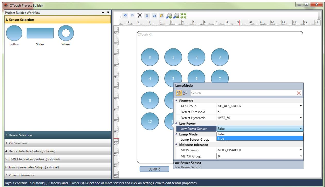
Figure 6-2 Adjusting Scan Rate of Low Power Sensor Using QTouch Project Builder
