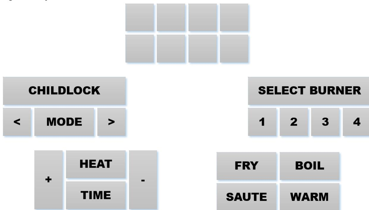
A total of eight physical sensor channels form the sensor panel. Lumping the same eight physical sensors can be reconfigured to create different logical sensors based on the functions that are needed in the current state.
