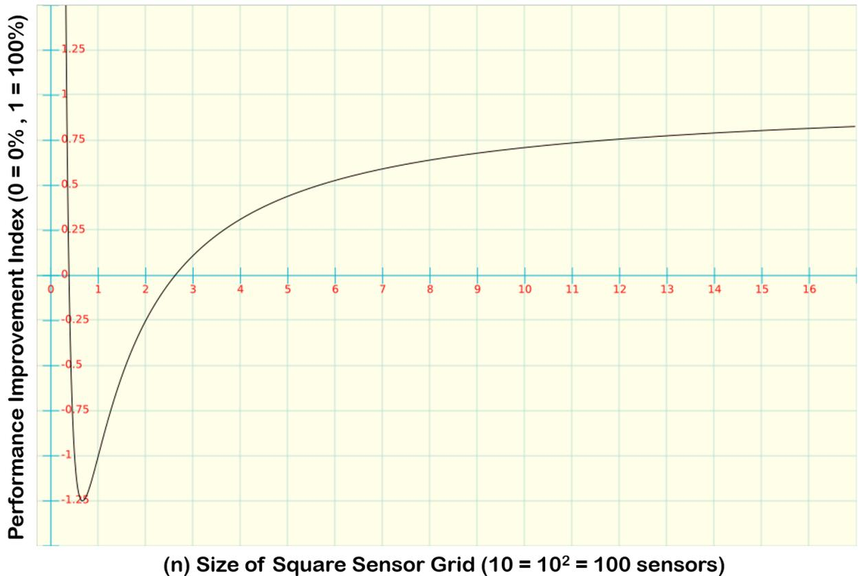
We can observe a dramatic improvement in the relative response time Smart Scan strategy as the number of keys increase in the system. For example, a touch panel with 36 keys, in a 6x6 configuration we can observe an improvement of more than 50% in the response time.
