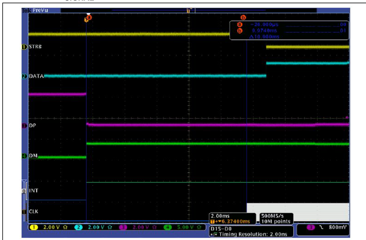
FIGURE 5: HUB WAKE-UP SEQUENCE WITH 10 MS DELAYED INT_N TRIGGERED CLOCK SIGNAL
