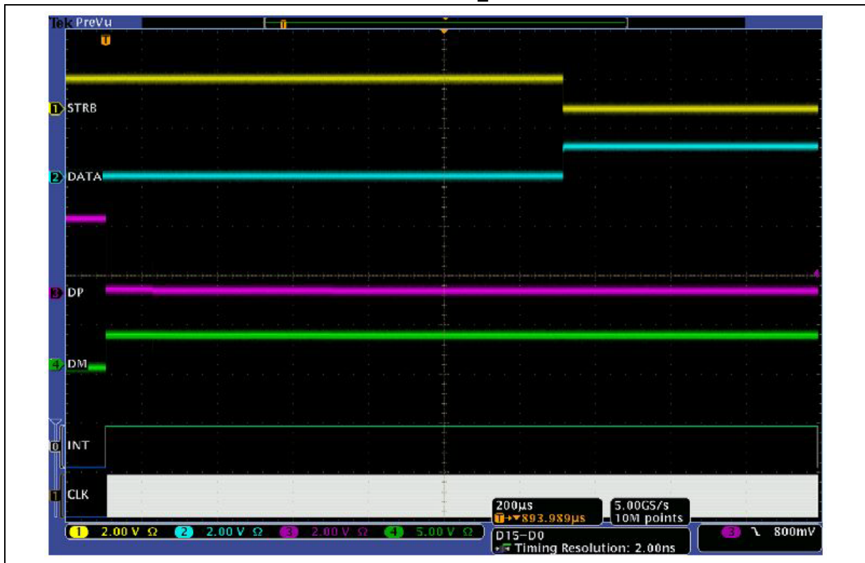
FIGURE 4: HUB WAKE-UP SEQUENCE WITH INT_N TRIGGERED CLOCK SIGNAL
