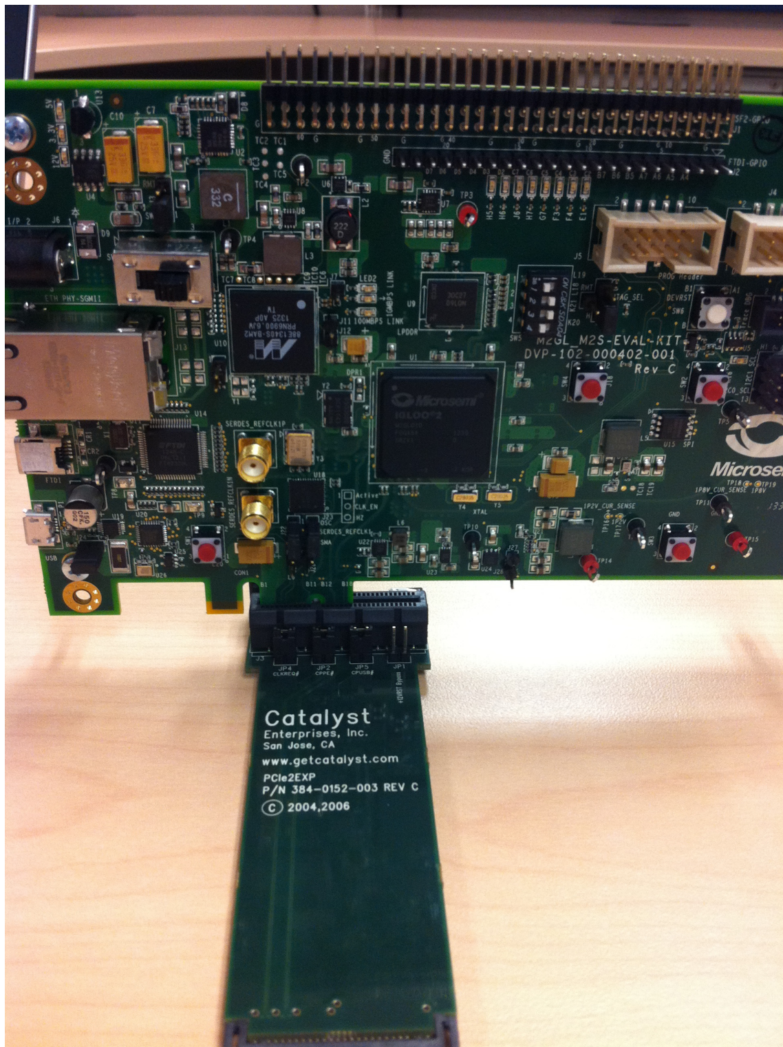
Figure 31 • Inserting the IGLOO2 Evaluation Kit PCIe Connector into the PCIe Adapter Card Slot
