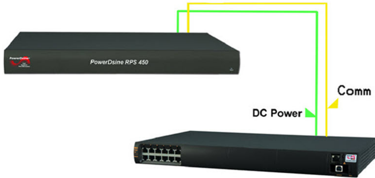
Figure 4-2. Secondary Midspan Power Backup
