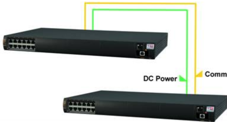
Figure 4-2. Secondary Midspan Power Backup
