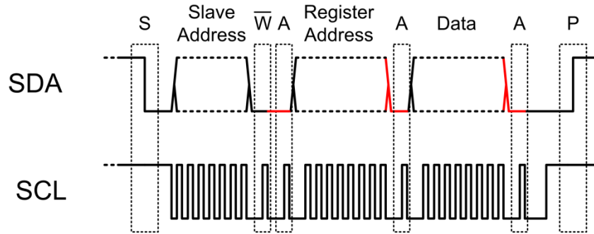
Figure 13. I 2 C Write Framing. Red Lines Indicate Slave Having Control of SDA.
