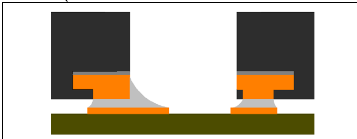
FIGURE 7: QFN/DFN STENCIL DESIGN
