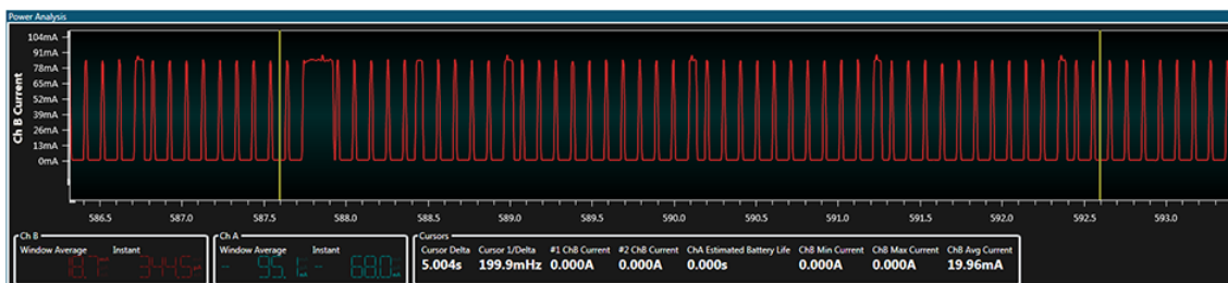
Figure 4-11. Automatic Power Save Mode Sequence
