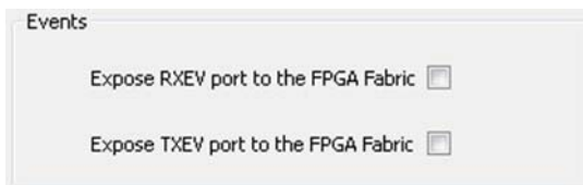
Figure 1-3 • RXEV and TXEV FPGA Fabric Interface Configuration
