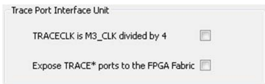
Figure 1-5 • TPIU FPGA Fabric Interface Configuration
