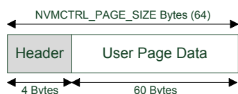
Figure 6-2. Internal Layout of An Emulated EEPROM Page
