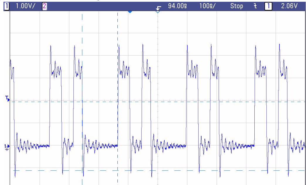
Figure 9-5. SDRAM CAS Signal for a 4-word Access with MMU
