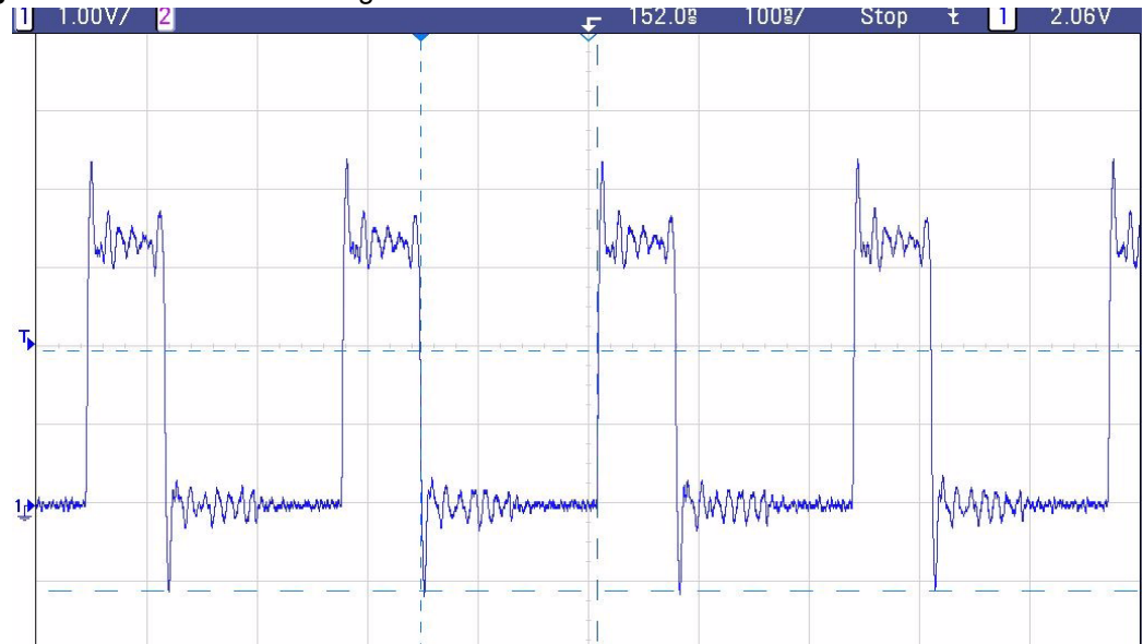
Figure 9-6. SDRAM CAS Signal for a 8-word Access with MMU
