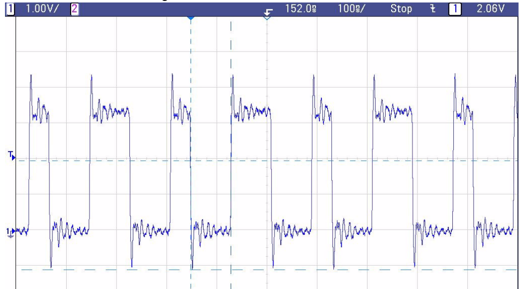
Figure 9-3. SDRAM CAS Signal for an 8-word Burst Access without MMU
