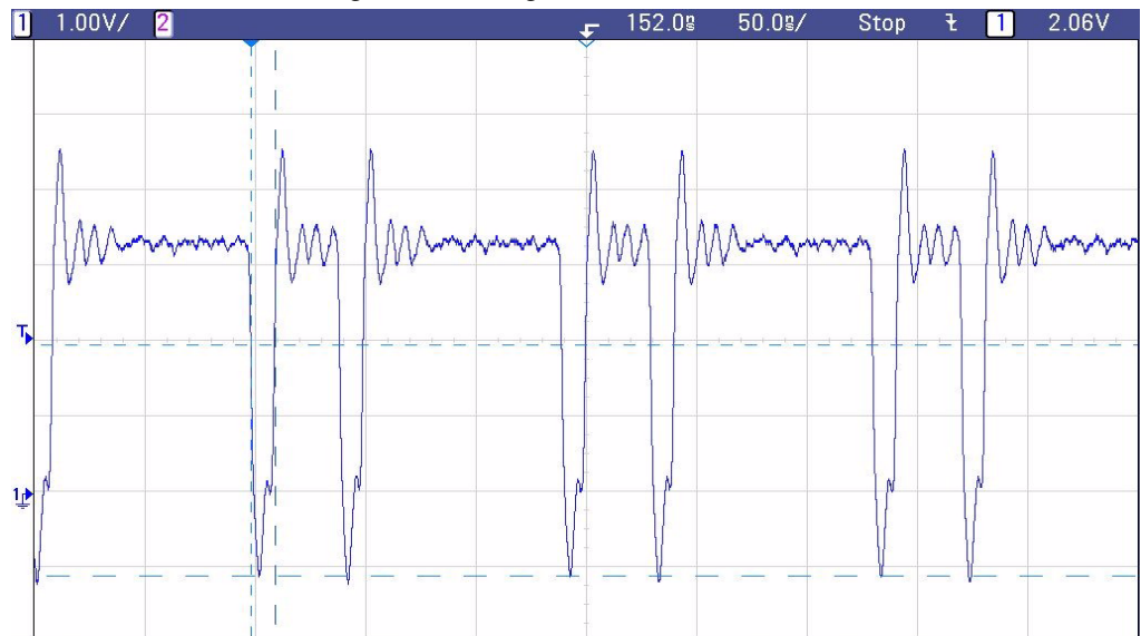
Figure 9-1. SDRAM CAS Signal for a Single Access without MMU
