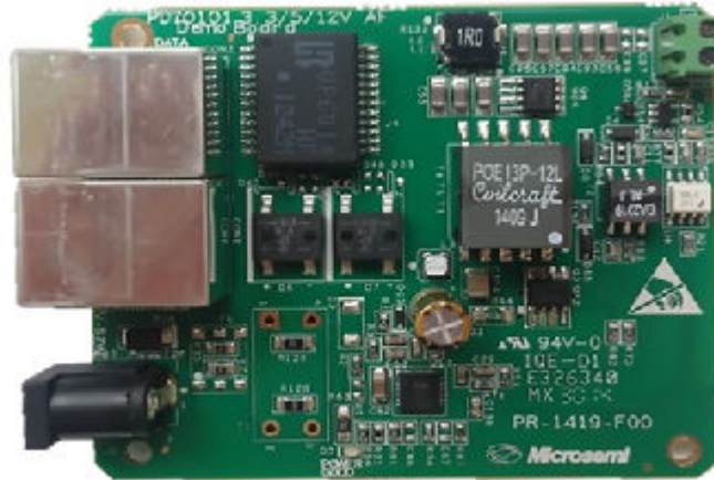
Figure 3-4. PD70101EVB6F Evaluation Board
