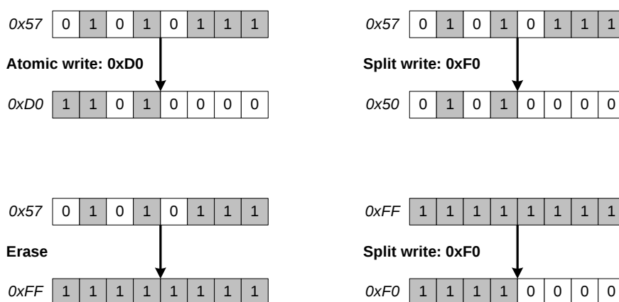
Figure 2-1. Atomic Write, Split Write and Erase Operations
