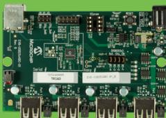
The EVB-USB2534BC is a four-layer RoHS-compliant evaluation board that utilizes the USB2534 to provide a fully functional 4-port high-speed hub with battery charging capabilities, IO bridging and FlexConnect to expand connectivity while lowering system BOM costs.
