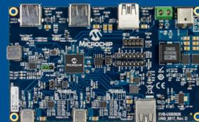
The EVB-USB7252 is a demonstration and evaluation platform for evaluating the USB7252C, a 4-Port SS/HS USB SmartHub on a 6-layer RoHS-compliant PCB. The EVB-USB7252 supports four downstream ports; two USB-C USB 3.2 Gen2 ports with integrated MUX and 2 Type A ports (1x USB Gen2, 1x USB 2.0).
