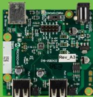
The board includes two downstream ports with individual port power control and battery charging support on each port and is targeted at 2-port, cost-sensitive applications.
