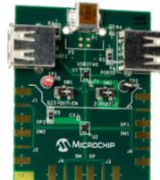
The USB3740 family of Hi-Speed USB switches were specifically designed to enable a range of applications to achieve single-port connectivity. Their design provides a substantial 1 GHz of bandwidth, allowing for the passage of robust USB 2.0 signals.
