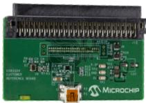
The USB333x family of Hi-Speed USB 2.0 transceivers delivers enhanced USB functionality for the portable market with support for the latest USB-IF Battery Charging 1.2 (BC 1.2) specification. This board provides an excellent complement to USB charging ports by enabling portable devices to negotiate up to three times the charging current compared to a standard USB port, resulting in faster battery charging.
