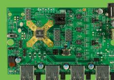
The Microchip USB4604 is a low-power, OEM configurable, MTT (Multi-Transaction Translator) USB 2.0 hub controller with four downstream ports and advanced features for embedded USB applications. The USB4604 provides the most package pins (48) allowing extensive IO bridging.
