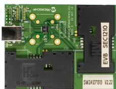
The EVB-USB2642 is a customer evaluation board that contains an ultra-fast USB 2.0 multi-format Flash media controller, a USB 2-port hub combo and a UCS81001 port power controller with charger emulation. This evaluation board includes a SMBus header interface to monitor I<sup>2</sup>C traffic from the USB to I<sup>2</sup>C bridge, as well as either an external I<sup>2</sup>C EEPROM or SPI Flash device for customized functionality.
