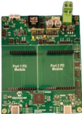
The USB7050P is a demonstration and evaluation platform of the USB7050P SmartHub on a 4-Layer RoHS-compliant Printed circuit Board (PCB). The 4-port USB7050P is compliant with the USB 3.2 Gen1 USB specification and supports SuperSpeed (SS), Hi-Speed (HS), Full-Speed (FS) and Low-Speed (LS) USB signaling. The board includes a PD interface socket (HAT) to add standard PD solutions for evaluation and test. Details on the interface itself is available on the Microchip website.
