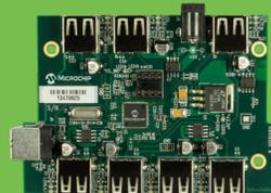
The USB2517 with MultiTRAK™ technology is a low-power, full-featured High-Speed USB 2.0 compliant hub with seven down-stream ports. With seven ports, sub-system expansion is maximized.
