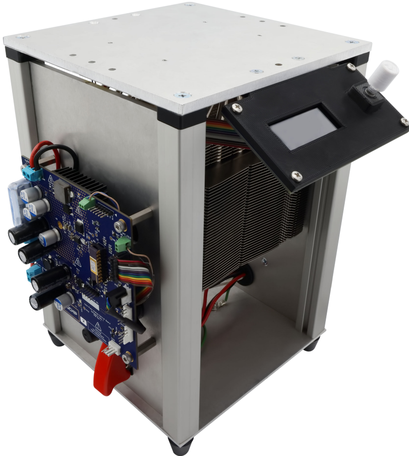
Figure 3-1. Completed Assembly of the Cold Plate
