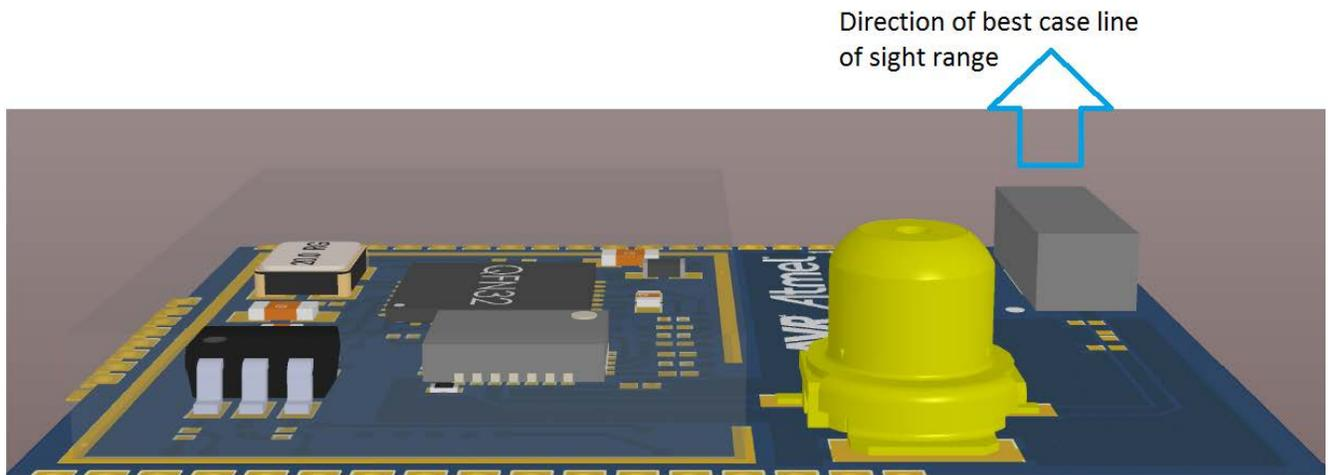
The Antenna in this module is designed to provide the best possible LoS range in the direction indicated in this illustration.
