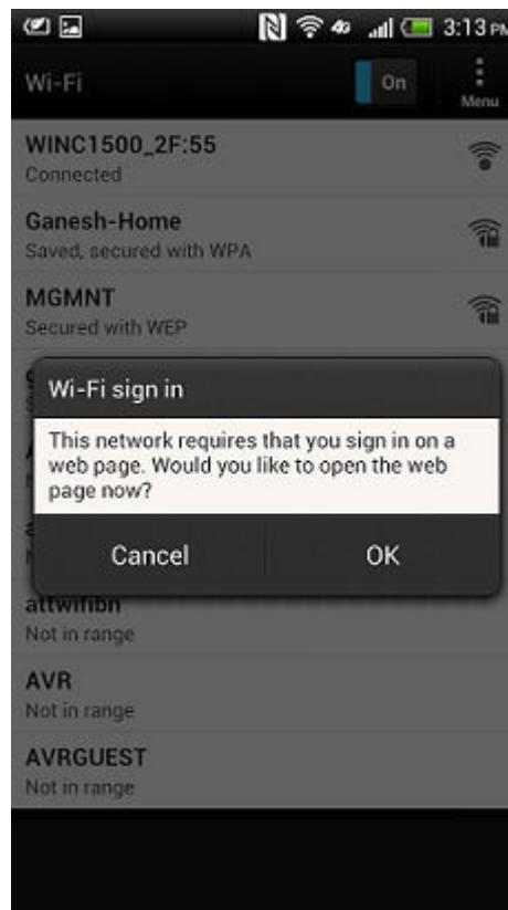
Figure 5-6. HTTP Web Triggering After AP Connection
