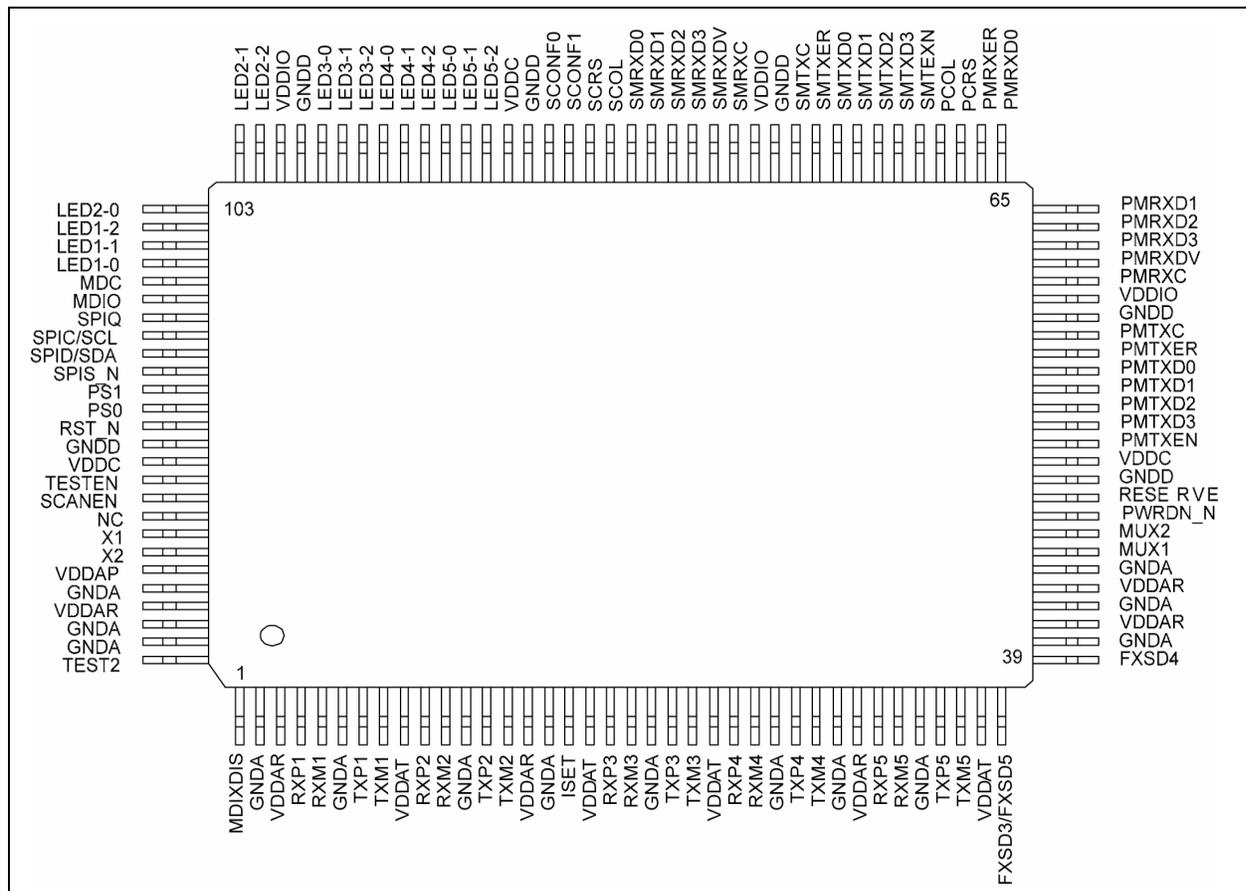
**FIGURE 1:** KSZ8995MA/FQ Pin Diagram.
