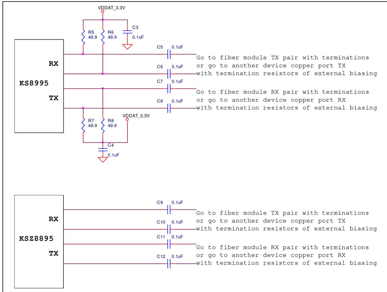
**FIGURE 4:** Connection Comparison for Fiber Module or Cap AC-Coupling with Two Copper Ports.
