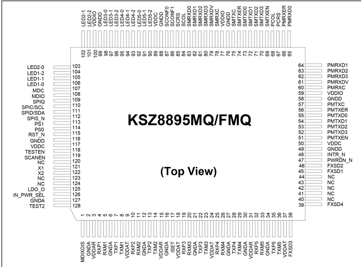
**FIGURE 2:** KSZ8895MQ/FMQ Pin Diagram.
