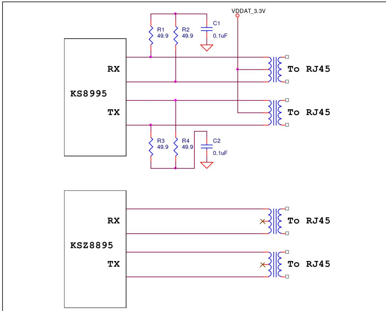
**FIGURE 3:** Connection Comparison for Copper Port.
