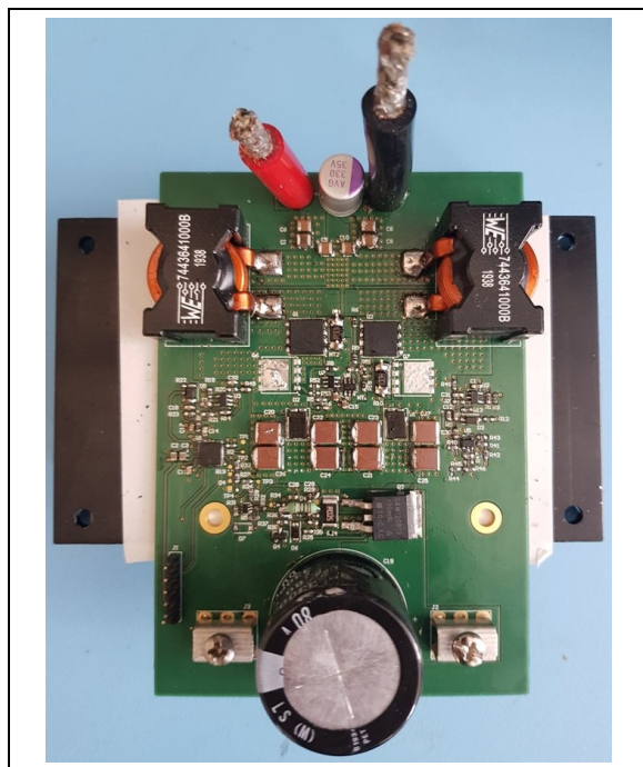
FIGURE 2: MCP19214/5 – 480W, 12V Battery-Powered, 120 mm x 85 mm PCB Prototype.
