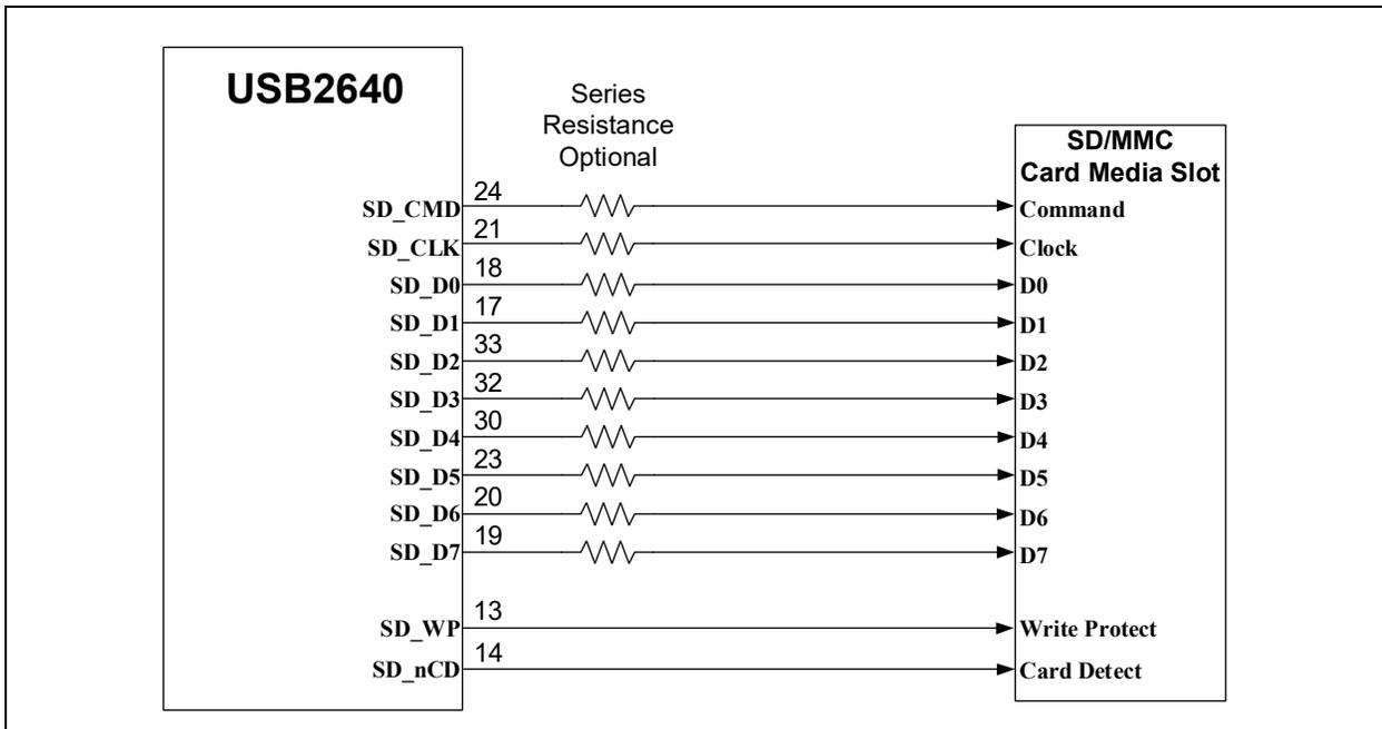
**FIGURE 5-2: EMMC (EMBEDDED MMC) MEMORY CONNECTIONS**
