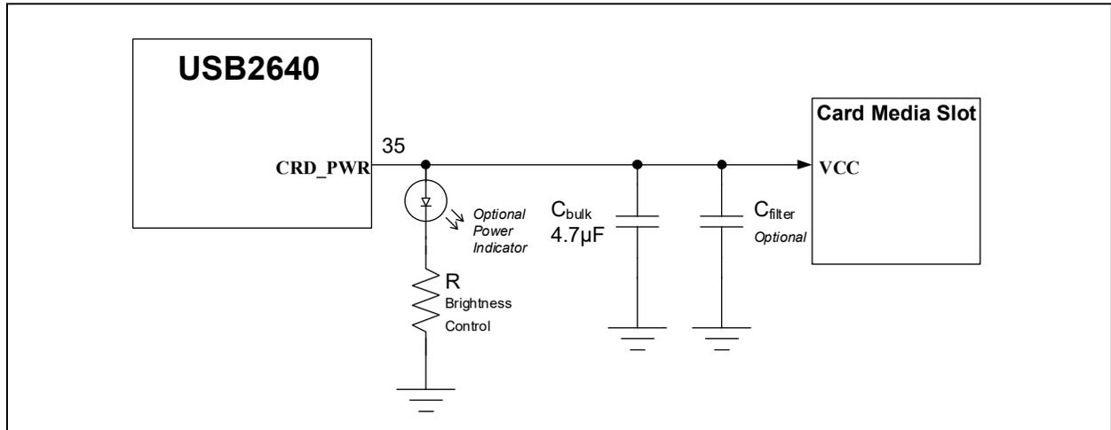
If the internal card power switch is not used, it is still recommended to use the CRD\_PWR pin to control the supply to the card media slot. This allows the internal logic of the USB2640 to reset power to the card during error recovery attempts.
