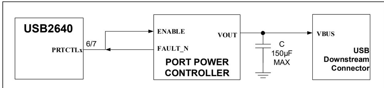
**Note:** The implementation, as shown in [Figure 4-3](#), assumes that the port power controller has an active-high enable input, and an active-low, open-drain style FAULT indicator. External polarity inversion through buffers or FETs may be required if the port power controller has different I/O characteristics.
