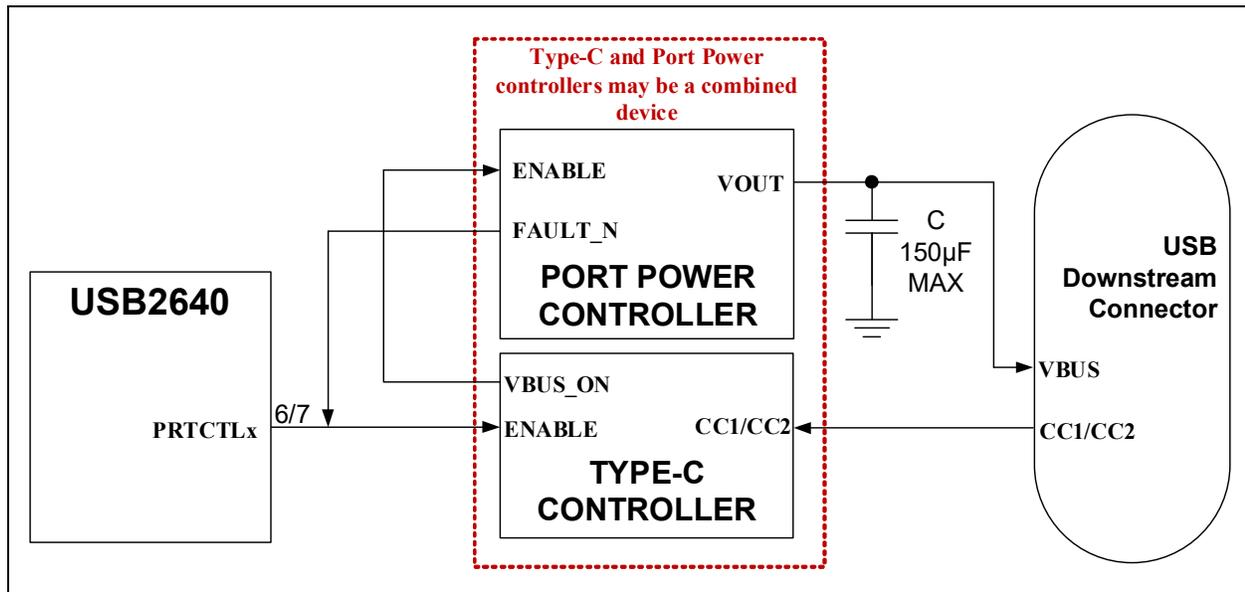
**Note:** The implementation, as shown in [Figure 4-4](#), assumes that the Type-C controller has an active-high enable input, and the port power controller has an active-low, open-drain style FAULT indicator. External polarity inversion through buffers or FETs may be required if the Type-C controller and/or port power controller has different I/O characteristics.
