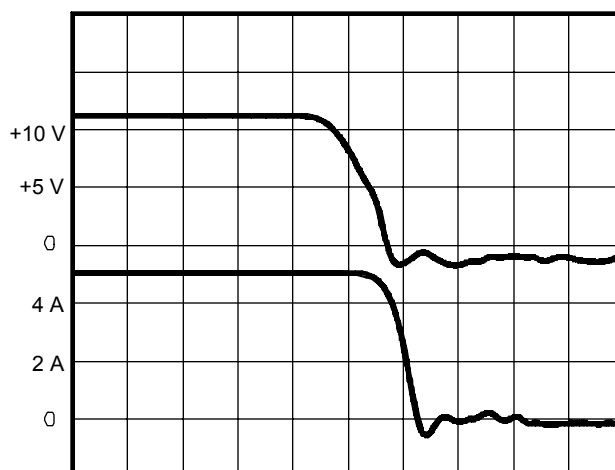
Figure 17. MOSFETS Turn-Off Waveforms. Upper Trace: Gate Voltage @ 100 ns/div. Lower Trace: Drain Current @ 100 ns/div.
