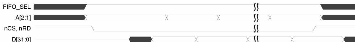
Figure 1.6 Burst Read Operation Using Direct FIFO Access
