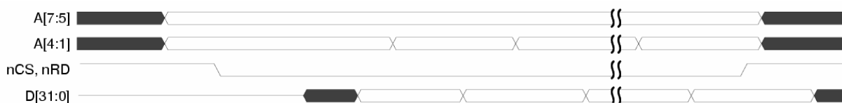
Figure 1.5 Simplified Burst Read Timing
