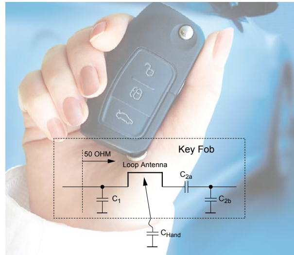
Figure 1. Influence of Human Hand's Capacitance on the Magnetic Loop Antenna
