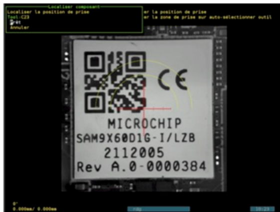
Figure 4-3. SAM9X60D1G SOM Pick & Place Operator View
