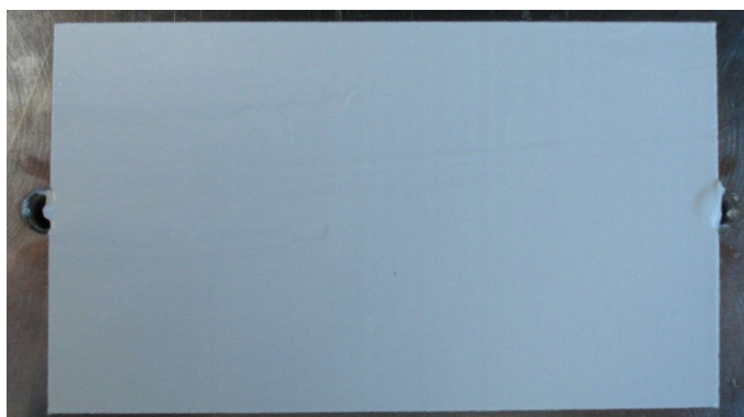
Figure 2-1. Grease on the Heat Sink Before Assembly
