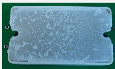
Figure 2-3. Grease on the Module After Disassembling
