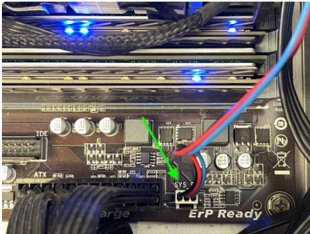
As it spins, a small magnet on the fan hub spins and triggers pulses from a Hall effect sensor. It's reporting **Current SYSTEM FAN Speed 1190 RPM**, which makes the BIOS happy.
