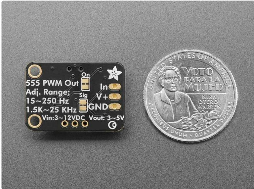
You can select between two 'ranges': approximately 1.4K~25 KHz or 1.4~250 Hz. The onboard trimmer pot will tune the actual output between those values. You can use a logic analyzer, oscilloscope, multimeter with frequency-counting, or even an audio input jack on a computer, to determine the precise value if you need more than a rough number. The output is a DC square wave, driven by a [74HC1G04](https://adafruit.it/1aOE) (<https://adafruit.it/1aOE>) buffer so it can sink/source up to 12.5mA.
