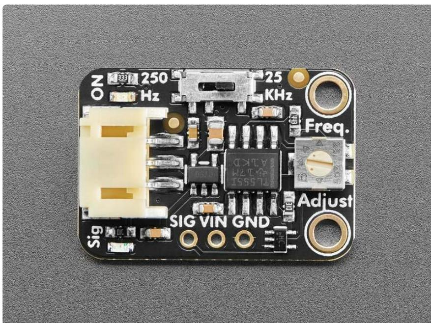
We originally came up with this idea when someone requested we make a 'PC Fan Dummy' board, that can generate a 100Hz signal for faking a PC fan's tachometer signal to a motherboard. But then we thought that sometimes we want a square wave for driving a piezo, or as an audio input, or to modulate an IR signal. So we made it a little more general-purpose.
