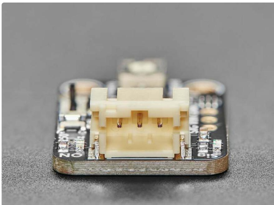
You can power the board from 3V to 12VDC, an onboard regulator will pin the input to the 555 and buffer to 5V max. That means that between 3V and 5V power, the signal peak will be at the same logic level as the power. Above 5V, the output will be pegged to 5V.
