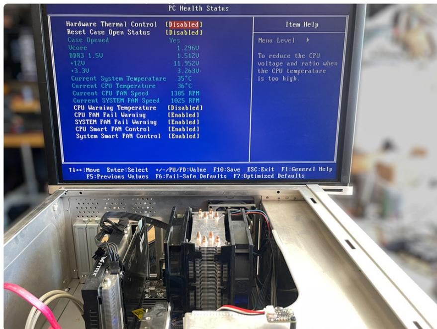
Here's how to use the 555 PWM Output STEMMA to trick your PC into thinking there's a fan running. This is useful when you've replaced the air cooling fans on your CPU or other parts of the system with liquid cooling radiators and pumps, such as a water cooled or oil cooled rig.
