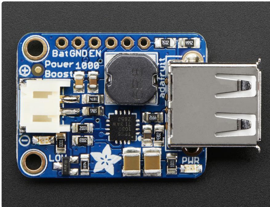
The PowerBoost 1000 has at the heart a [TPS61030 boost converter from TI \(https://adafruit.it/dLY\)](https://adafruit.it/dLY). This boost converter chip has some really nice extras such as low battery detection, 4A internal switch, synchronous conversion, excellent efficiency, and 700KHz high-frequency operation. Check out these specs!
