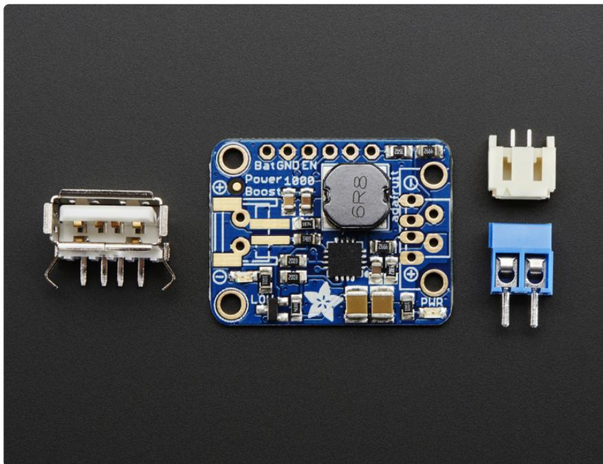
If you are powering your project from USB, solder the USB A jack in (a 3-minute soldering task). Then choose either JST for input (JST is often used for our Lilon batteries, but the connector is only rated for 2A) or a terminal block.
