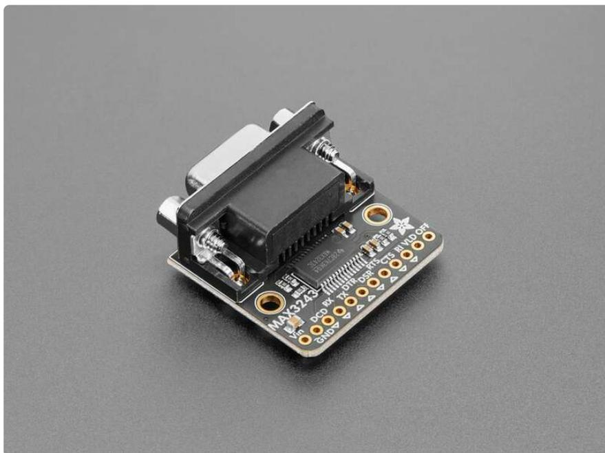
If you want to use a microcontroller or microcomputer to chat with an RS-232, then thankfully, all you need is a serial port / UART (something just about any microcontroller has) and a level shifter. The level shifter is required because while most UARTs are 0-3.3V or 0-5V logic level, RS-232 requires +6 to +10V, yep the signal voltage goes negative! That means a specialized shifter is required to generate extra high and low voltages and safely convert the logic levels.
