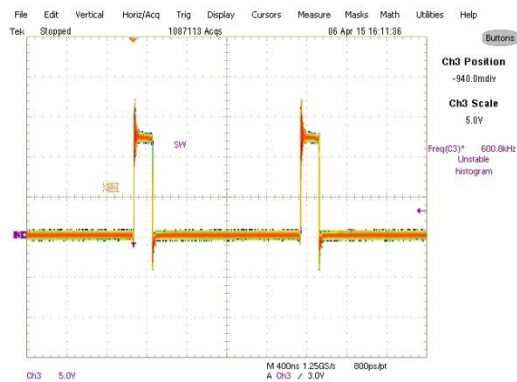
Figure 45: Inductor node at 25A load Ch 3 :SW node
