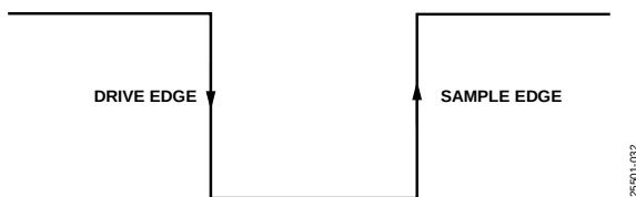
Figure 34. SPI Mode 3 SCLK Edges
