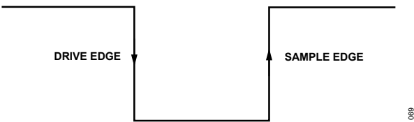
Figure 65. SPI Mode 3, SCLK Edges
