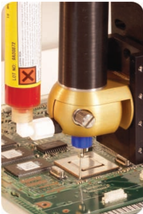
TS5000DMP - performing underfill.
