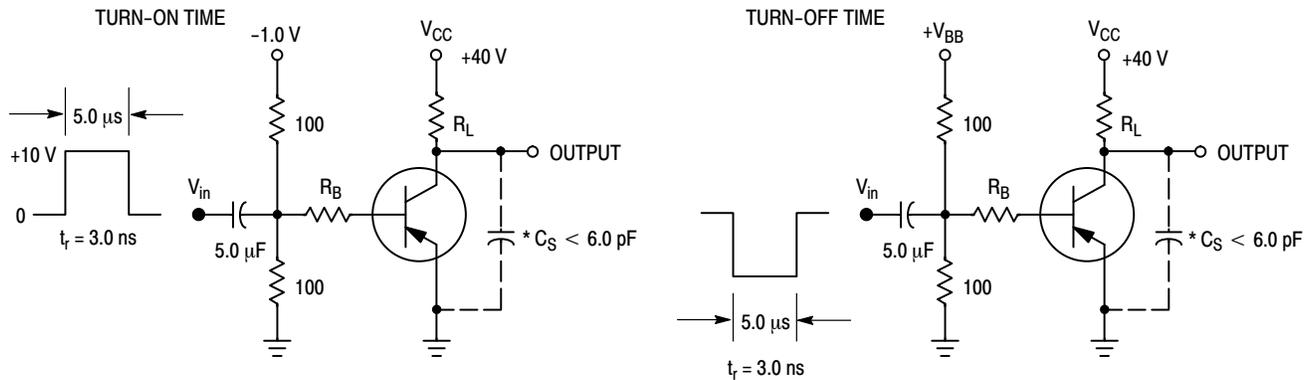
\*Total Shunt Capacitance of Test Jig and Connectors For PNP Test Circuits, Reverse All Voltage Polarities
