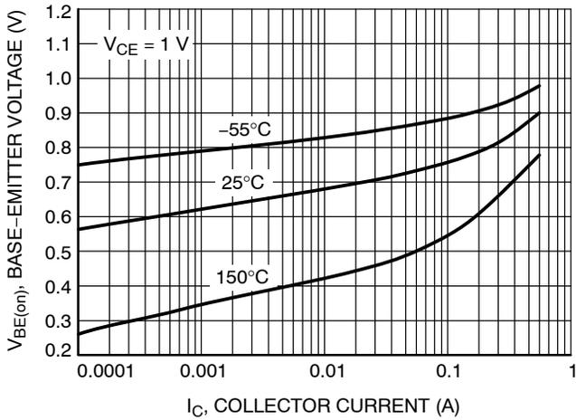
**Figure 8. Base Emitter Voltage vs. Collector Current**
