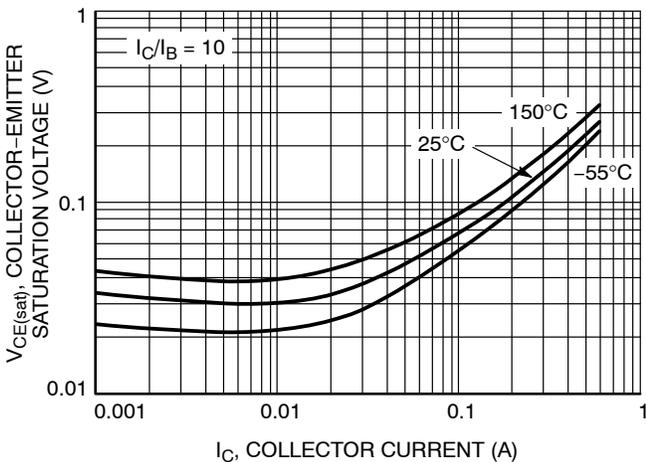
Figure 6. Collector Emitter Saturation Voltage vs. Collector Current
