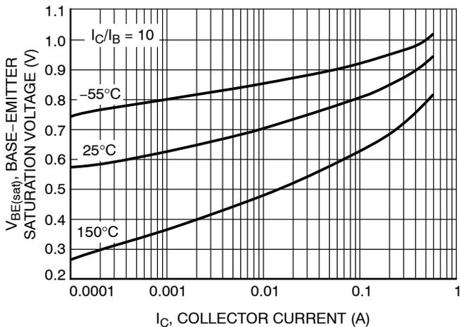
Figure 7. Base Emitter Saturation Voltage vs. Collector Current
