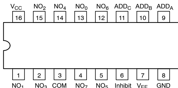
Figure 1. Pin Connection (Top View)
