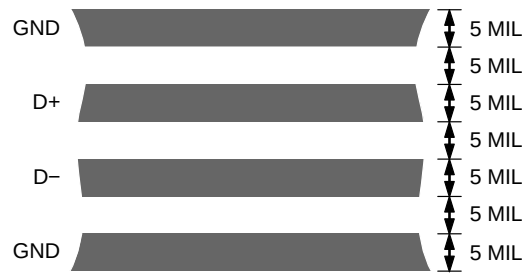
Figure 22. Typical Arrangement of Signal Tracks
