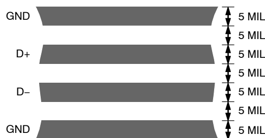
Figure 22. Typical Arrangement of Signal Tracks
