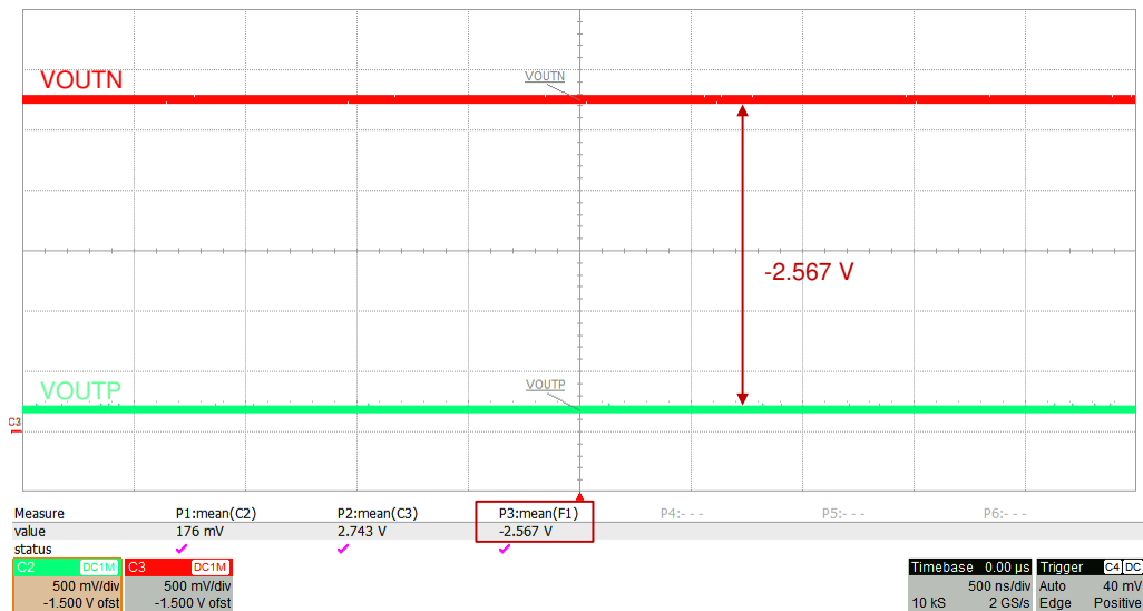
Figure 7-4. Typical Fail-Safe Output of the AMC3311
