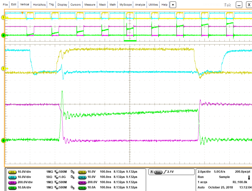
Figure 8-6. SiC MOSFET Switching Waveforms
