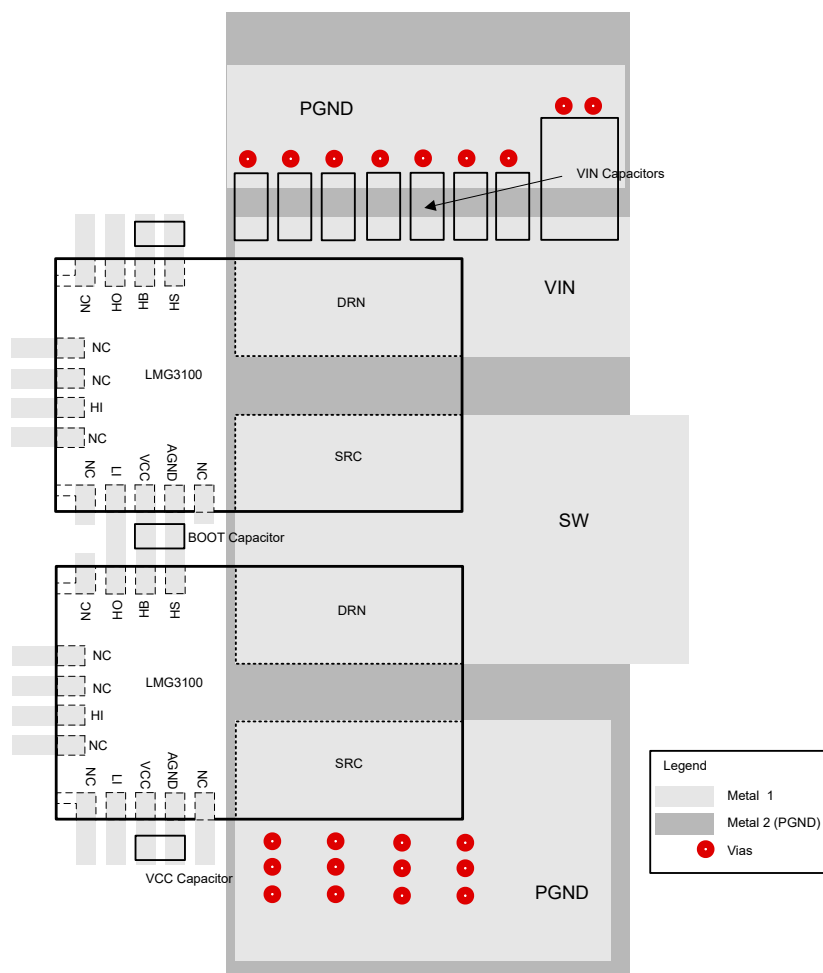
Figure 8-6. External Component Placement (Multi Layer Board)
