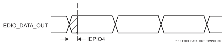
Figure 6-76. PRU-ICSS IEP Digital IOs Timing Requirements
