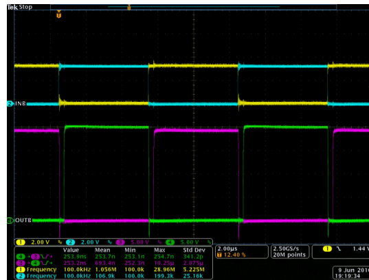
Figure 8-5. Bench Test Waveform for INA/B and OUTA/B
